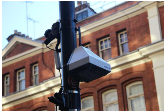
AQMesh pod installed on a lamppost with mains power supply. Credit: ACOEM Air Monitors.
